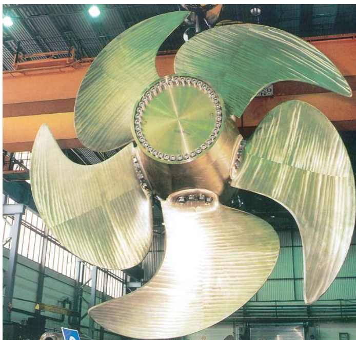
5-bladed control pitch propeller for a container
