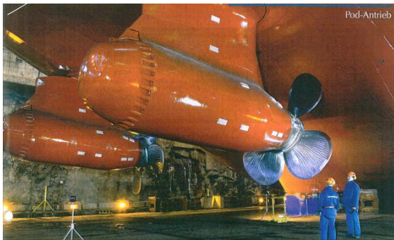
Electric 'Azipod' propulsion
