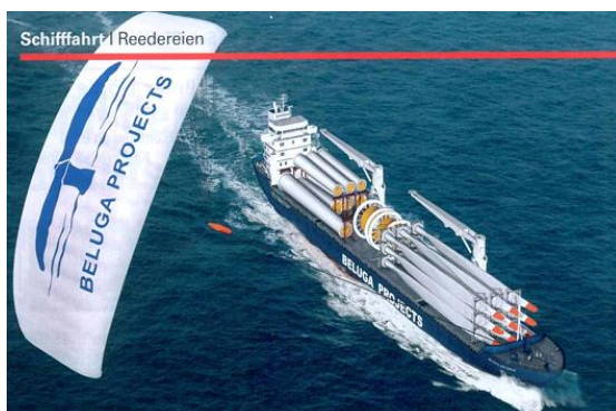
Left: SkySail – only suitable for „auxiliary propulsion“!
