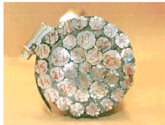
Design of the CASAR Powerplast wire rope (cross-section of the wire rope)
