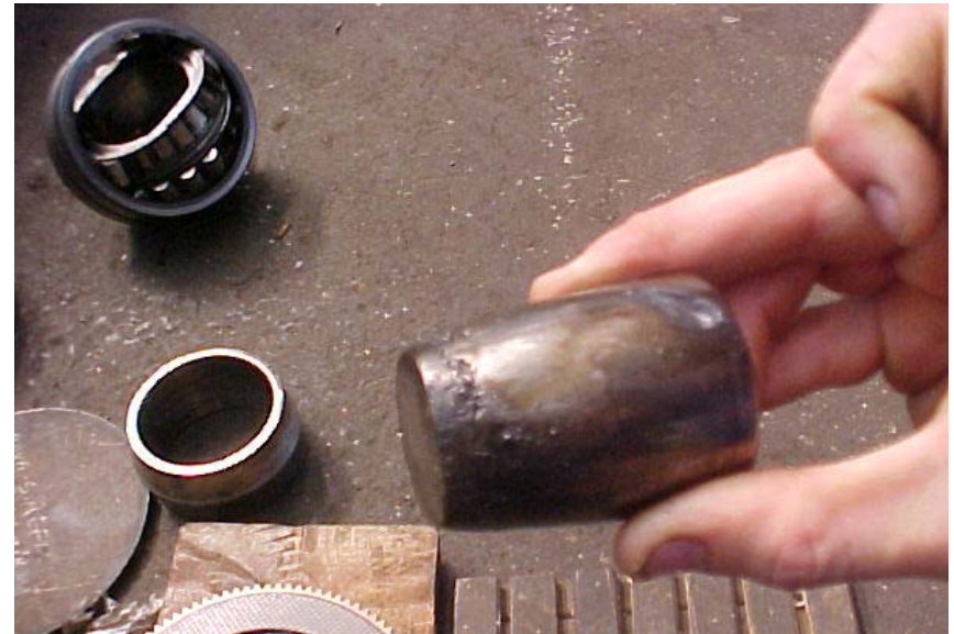
Damaged roller body
