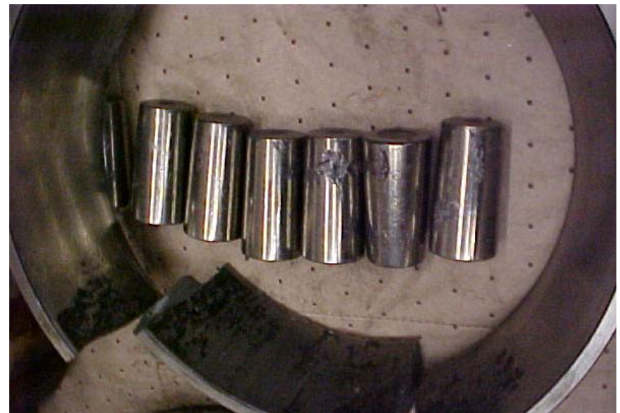
Broken ball race and roller bodies of a thrust bearings
