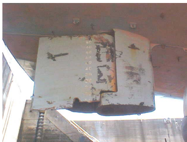
Caused by a crack in the geometrical notch the lower section of a rudder has been lost at sea.
