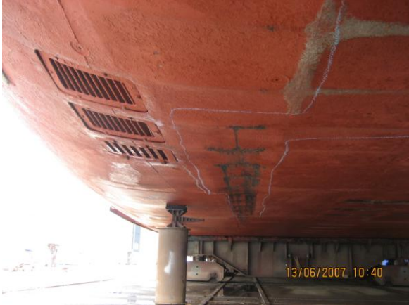
provisional supports in the repair area
