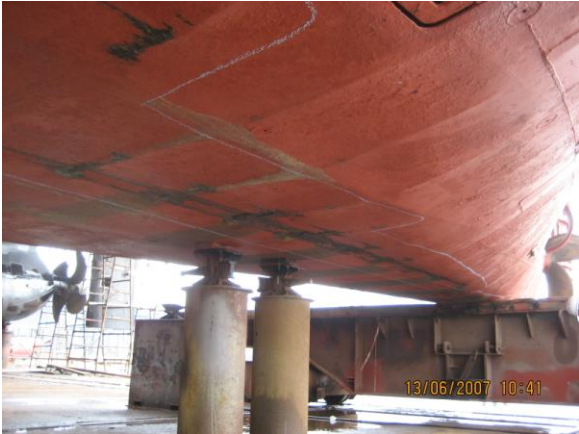
provisional supports in the repair area
