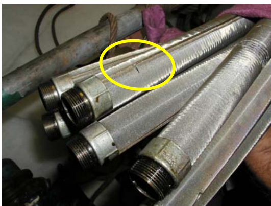
Damage to filter candles due to improper storage
