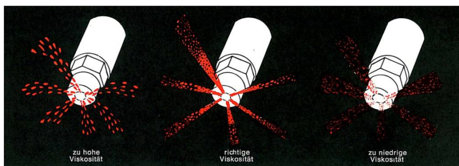
Influence of the fuel viscosity on the injection quality
