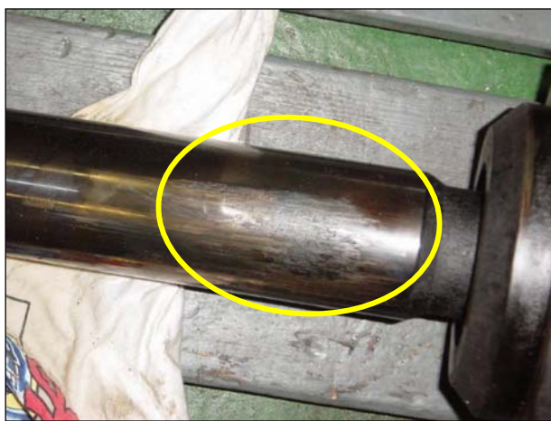
Fuel pump plunger with score/seizing marks
