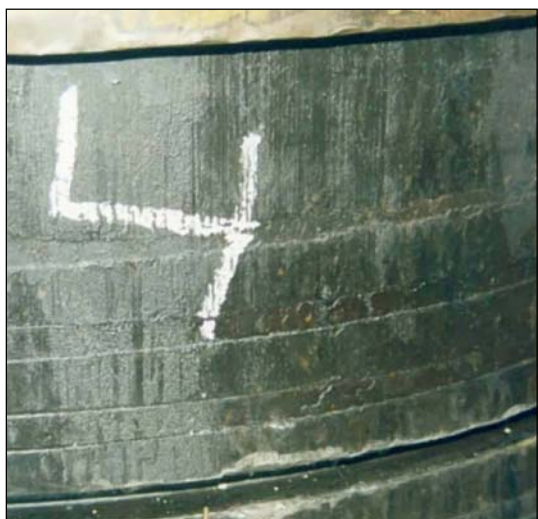
Piston crown with seized rings
